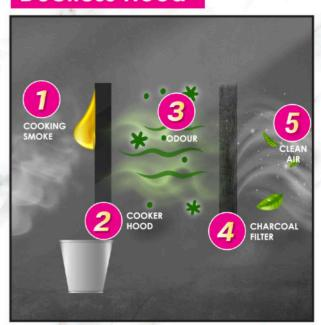
If you not able to make a coring hole in your kitchen wall, you'll need to install the hood as recirculation system. It consists of charcoal filter that function to filter the odour and release clean air back in your house.
