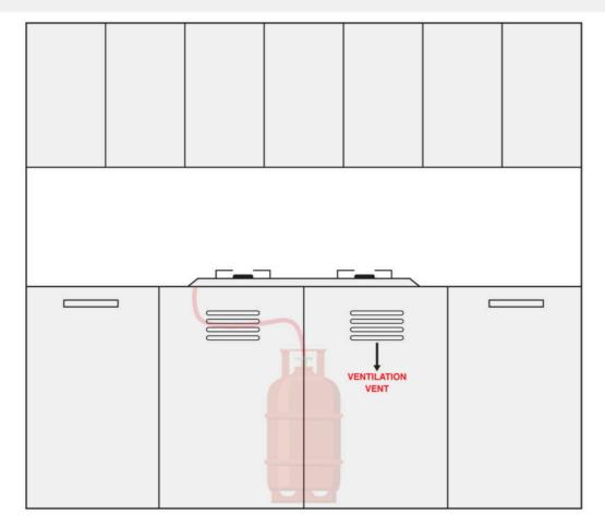
When installing a gas stove into a built-in cabinet, **MAKE SURE** there is sufficient space for proper ventilation within the cabinet to prevent any potential hazards. It is highly recommended to install a ventilation vent on the cabinet door for added safety.
