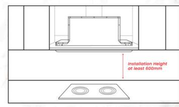
**STEP 5:** Kindly take note that the installation height between Cooker Hood and Stove, the recommended installation height is **around 600mm.**
