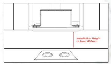
STEP 5: Kindly take note that the installation height between Cooker Hood and Stove, the recommended installation height is around 600mm.
